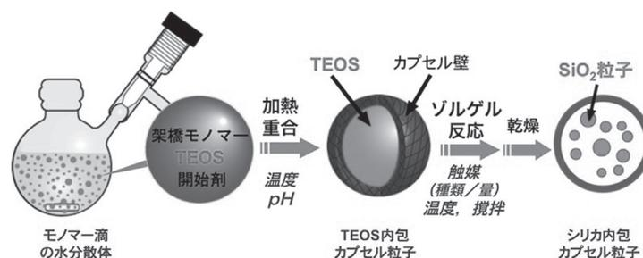
Scheme 1 Scheme of one-pot synthesis of polymer capsules with silica particles
