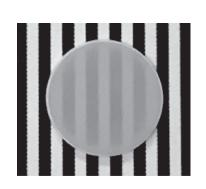
Fig. 7 Photograph of SrHfO<sub>3</sub> ceramic.  $11 \text{ mm}^{\phi} \times 1.1 \text{ mm}^{t}$
