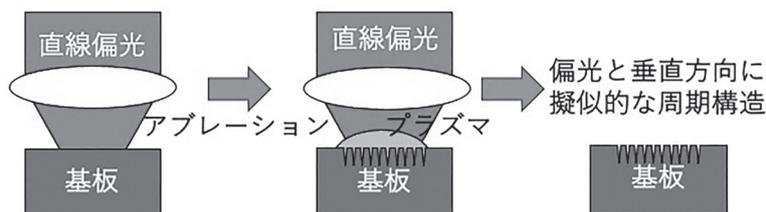
Fig. 2 Schematic of the laser-induced periodic surface structure fabrication method.
